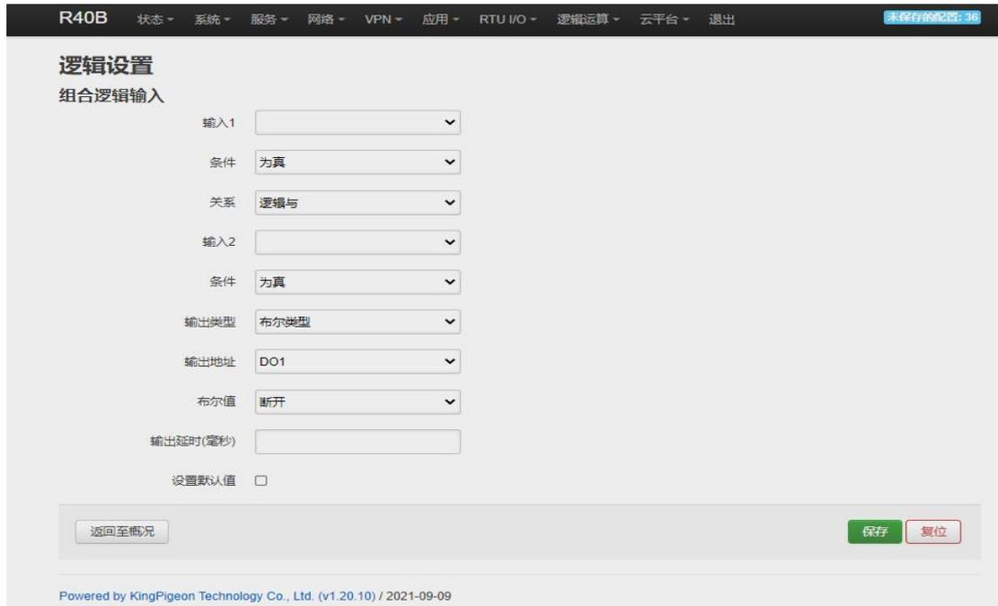
The logical operation function can link the local device I/O (digital input and output, analog input) with the Modbus slave I/O (slave device register), combine them at will as required.
